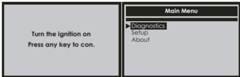
6. Press ENTER to confirm. A sequence of messages displaying the OBD II protocols will be observed on the display until the vehicle protocol is detected
