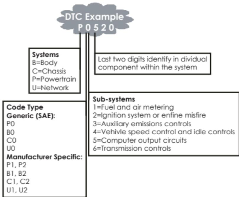
**Figure 1-2: Explanation of a diagnostic trouble code.**
