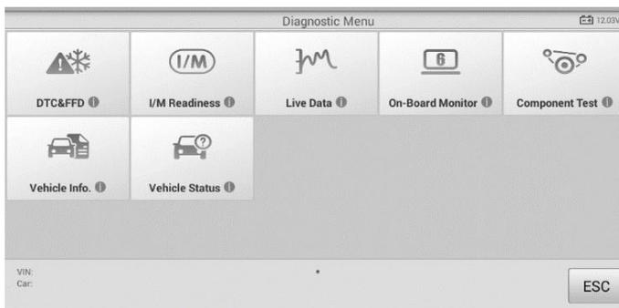
**Figure 4-17 Sample OBDII Diagnostic Menu**
